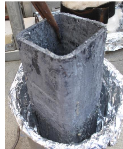
Thermomechanical response of heated FCI in PbLi (Hypertherm)
